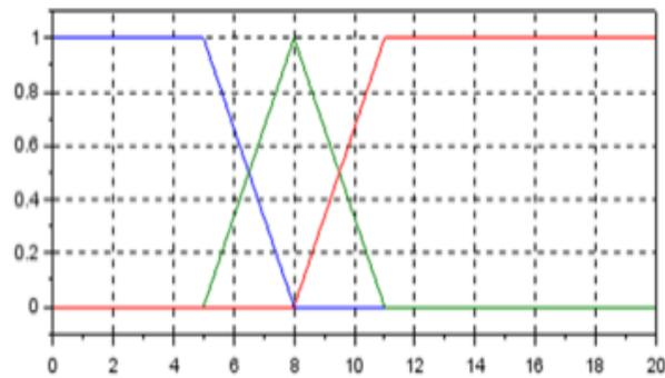
Figure 3. Membership function of YF-S201 flow sensor
