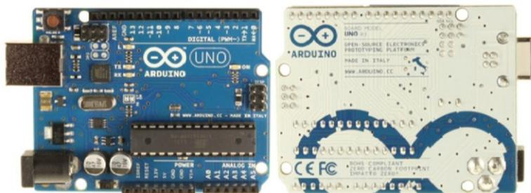
Gambar 1 Papan Arduino Uno R3 [6]
