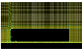
Fig 5. Meshing bluff body without adding Diffuser
