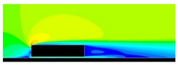
Fig 9. Contour Velocity In Bluff Body Model Without Diffuser Addition
