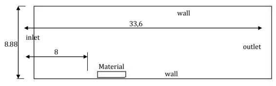
Fig 1. Dimensions and boundary conditions of numerical simulations
