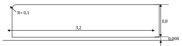
Fig 3. Bluff body Without Additional Diffuser
