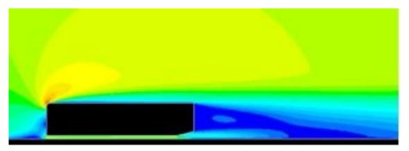
Fig 8. Contour Velocity On Bluff Body Model With Diffuser Addition
