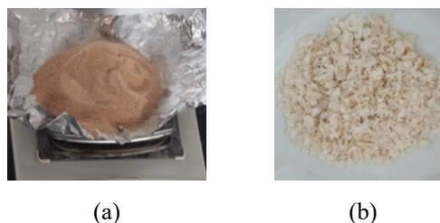
Figure1. Sampel (a) Sago Fiber, (b) Cellulose Extraction Results
