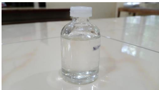
Figure 1. DES solution at a Cholin Chloride-Urea ratio of 1:2
