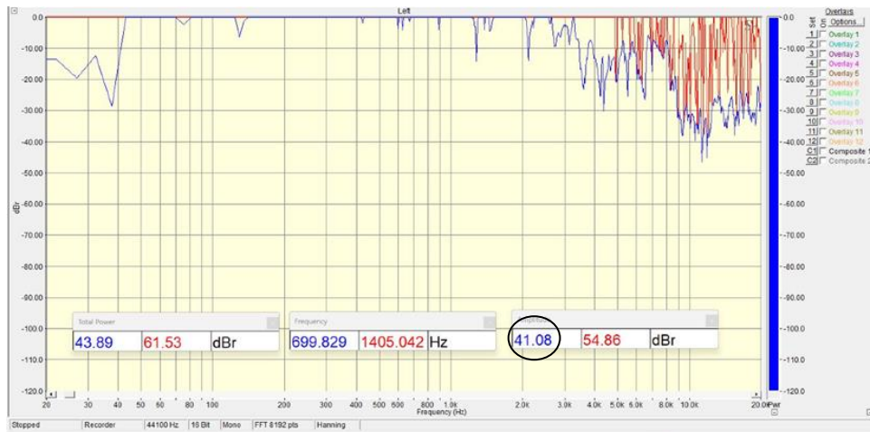
Figure 9. Spectra plus software analysis of the superposition of 2 nd gamelan barung and gamelan peking audio waves.
