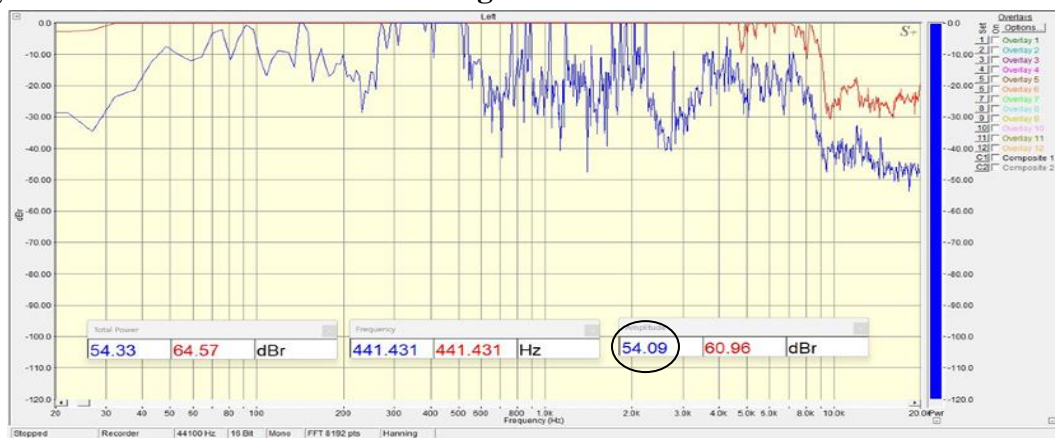
Figure 1. Spectra plus sound card software analysis of the saron demung wave.
