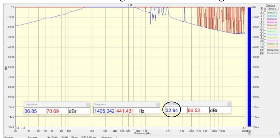
Figure 10. Spectra plus software analysis of the superposition of 2 nd gamelan barung and gamelan demung audio waves.
