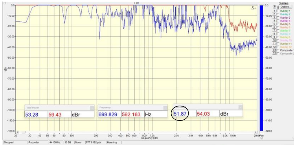
Figure 5. Spectra plus software analysis of gamelan peking audio.
