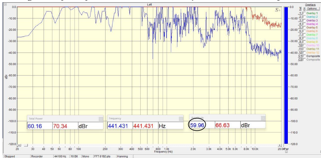
Figure 2. Spectra plus sound card software analysis of the saron demung gamelan with the same audio file.
