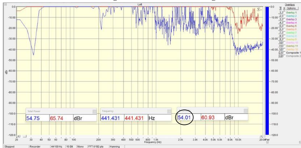
Figure 7. Spectra plus software analysis of the superposition of 1 st gamelan barung with gamelan demung audio waves.
