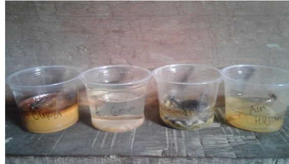
Figure 1. Immersion specimen media without coating
