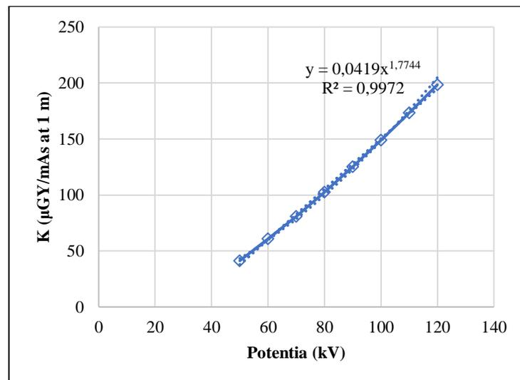
**Figure 2.** X-ray radiation output graph
