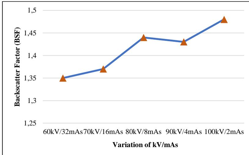
**Figure 4.** The relationship between variations in the value of kV on the backscatter factor
