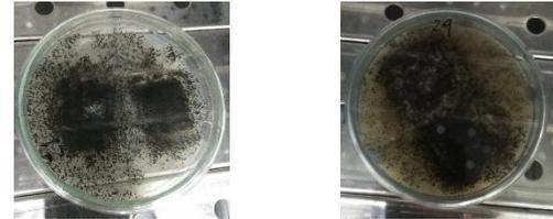
**Gambar 6.** Hasil biodegradasi H-14 bioplastik (a) 0% ZnO (b) 3% ZnO
