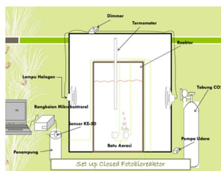
Figure 1. A Set of photobioreactor
