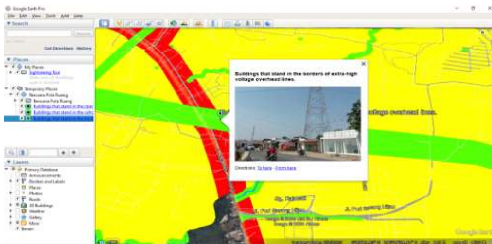
Figure 5. Map of Buildings That Stand in The Borders of Extra-High Voltage Overhead Lines.
