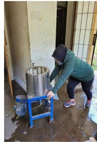
**Figure 3.** Posture When Moving the Modified Cilembu Sweet Potato Washing Machine
