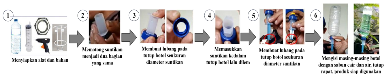
Figure 1. Steps to make a simple automatic hand soap dispenser product.
