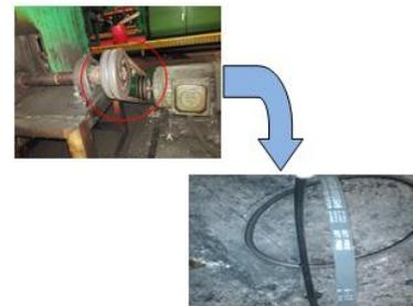
**Gambar 9.** Proses Pelepasan *Van Belt*
