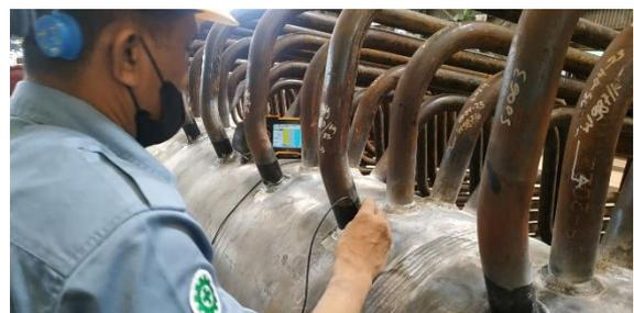
**Gambar 4** proses uji ultrasonik
