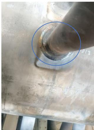
**Gambar 2** hasil pengelasan *stube to header*
