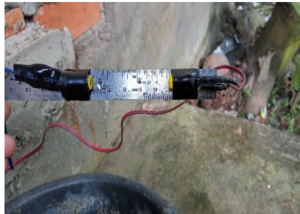
Figure 9. placing the sensor distance using the ruler
