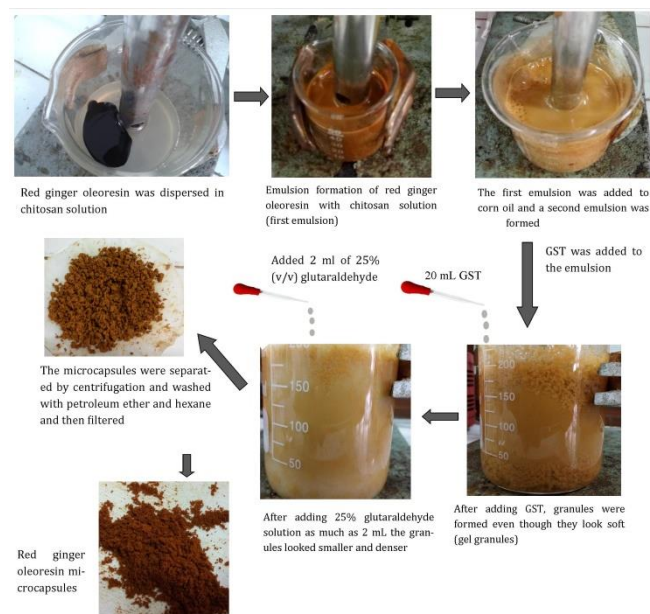
Fig. 2. The emulsion crosslinking method for encapsulation of red ginger oleoresin
