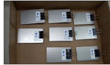
Fig. 1. JIS G-3141 . metal sample
