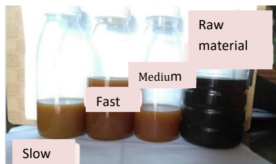
Fig. 2. The product oil of despicing process at different mass flow rate.
