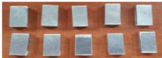
Fig. 1. AA 5052 which has been cut to a size of 5 mm x 10 mm x 20 mm
