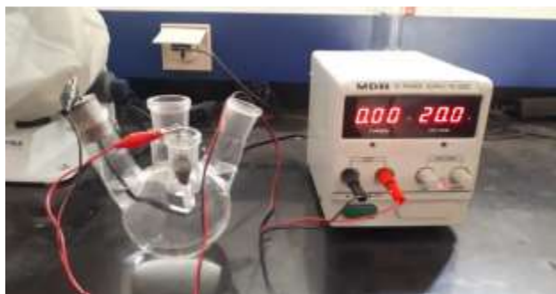
Fig. 2. EPD process using DC power supply
