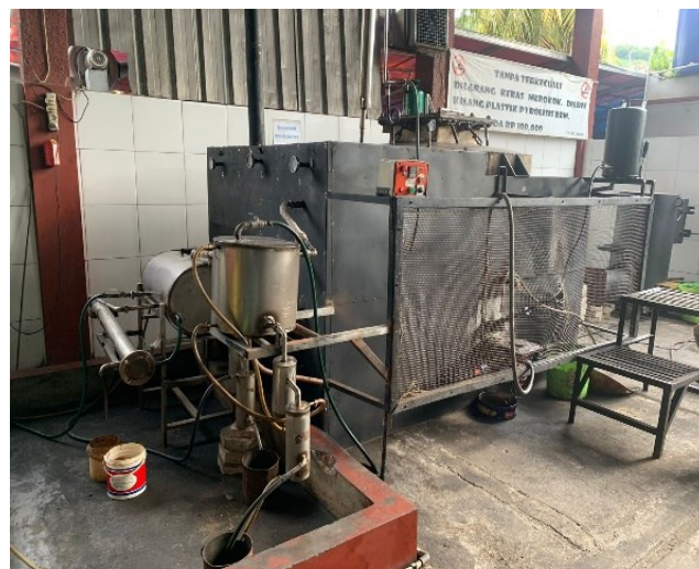
Fig. 1. Pyrolysis Equipment Scheme for Treating Plastic Waste
