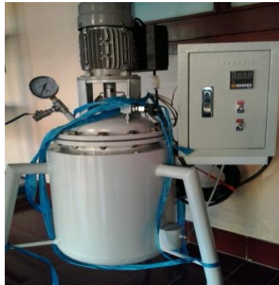
Fig. 1. Evaporation for processing UBC of coal
