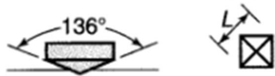
Fig. 4. Indenter of the Vicker's hardness tester
