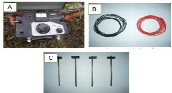
Fig. 1. Soil Resistance Measuring Instrument; (A) Meter resistance, (B) Copper cable, (C) Pin for plugging into the ground
