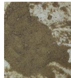
Figure 3. Na-alginate from Sargassum binderi (100 mesh)
