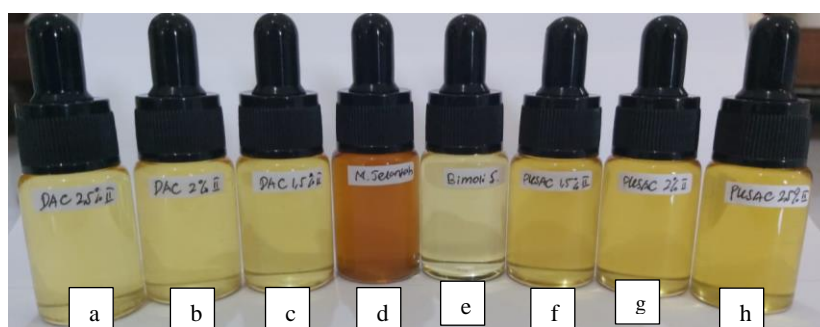
Figure 1. Waste cooking oil after purification using PKSAC-AC260 as well as DAC and control cooking oil. a (DAC 2.5%); b (DAC 2%), c (DAC 1.5%); d (waste cooking oil); e (control cooking oil); f (PKSAC-AC260 1.5%); g (PKSAC-AC260 2%); h (PKSAC-AC260 2.5%)
