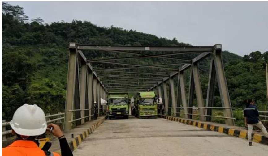
Figure 15. The process of testing the static loading of the Citanduy Bridge
