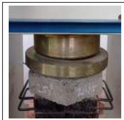
Figure 5. Paving Block Compressive Strength Test
