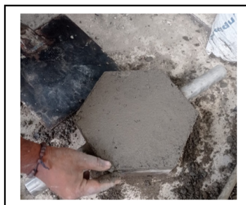
Figure 3. Paving Block Making Process
