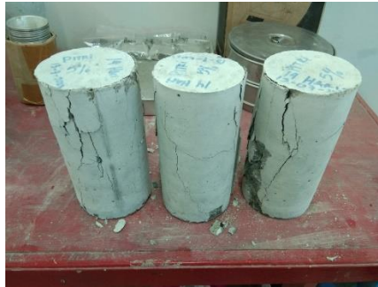
Figure 5. Crack pattern of 5% cockle shell powder specimen
