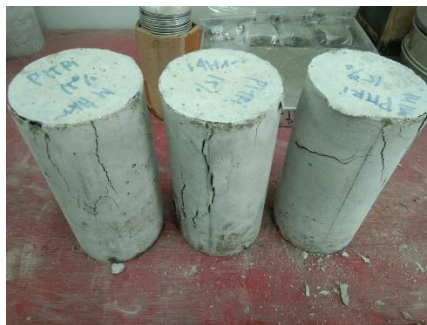
Figure 6. Crack pattern of 15% cockle shell powder specimen
