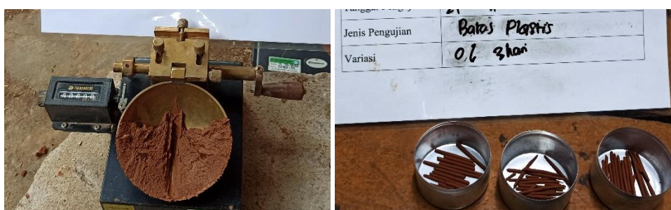
Figure 8. Atterberg limit test
