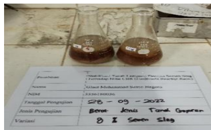
Figure 4. Specific Gravity Test
