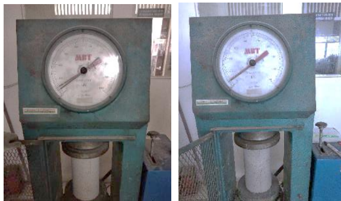
Figure 6. Concrete compressive strength testing in the laboratory
