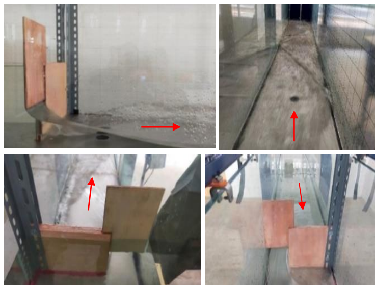
Figure 8 Water Flow Conditions When The Sluice Gate is Opened ( a = 13 cm)
