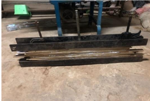
Figure 2. Gluing Process of Laminated Bamboo Beams
