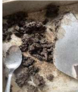
Figure 3. Soil mixture with fly ash based geopolymer
