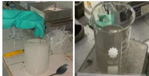
Figure 4. Preparation of Alkaline Activator (NaOH and Sodium Silicate)
