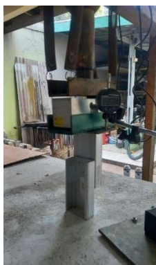
Figure 6. Setting-Up Shear Test of Light Steel Joints
