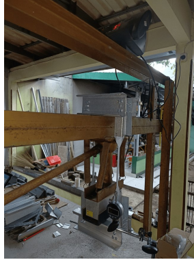
Figure 4. Tensile Strength Testing Set-Up
