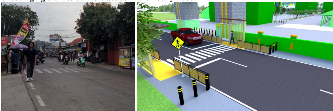
Figure 6. Existing Condition & 3D Design of Segment 2 Crossing Facility
