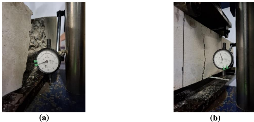
Figure 6. (a) Normal Concrete Block Collapse, (b) Fiber Concrete Block Collapse
