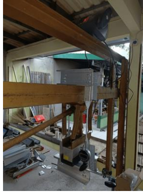
Figure 4. Tensile Strength Testing Set-Up
