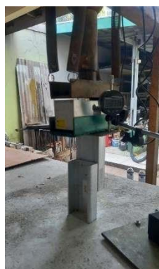
Figure 6. Setting-Up Shear Test of Light Steel Joints
