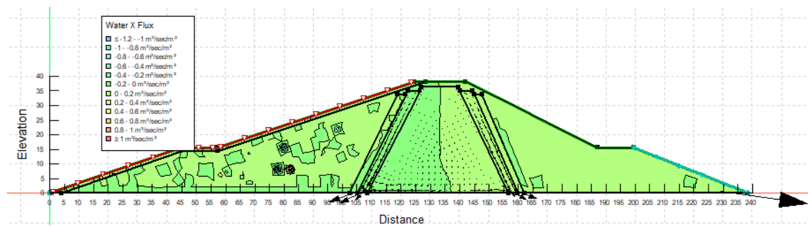
Figure 7. Water Seepage in Transient Conditions at Flood Water Level in 30 Days
