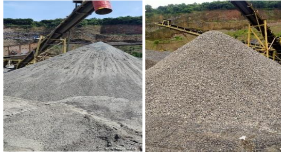
Figure 1. Natural Aggregates and Nickel Slag Aggregates
