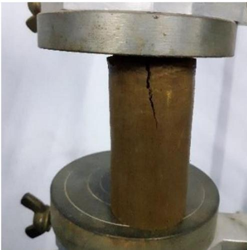
**Gambar 13.** Pola Keruntuhan Tanah Asli
