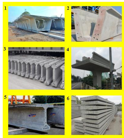
Gambar 3. Box Girder (1), PC-U Girder(2), PC-I Girder (3), Pier Head (4), PC-T Girder(5), Voided Slab (6)
