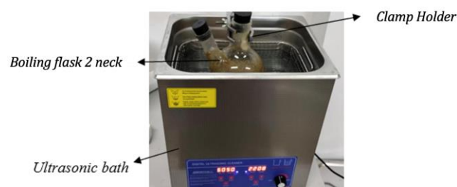
Figure 1. Ultrasonic-assisted extraction setup
