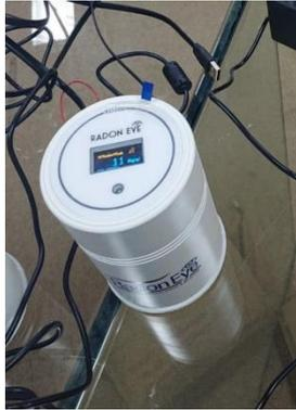
Gambar 6. Sensor gas radon
