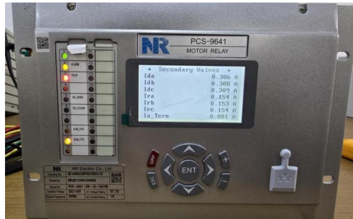
Figure 7. Relay Protection Device Id& Ir Sampling and Trip Action LED Lit
