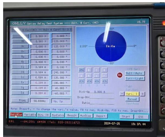
Figure 10. Relay Tester Display on Current Injection Process I_{a,b,c} is Current on the Terminal Side I_{x,y,z} is Current on the Neutral Side
