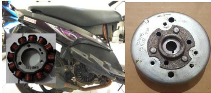
Gambar 2 Alternator sepeda motor mio sporty
