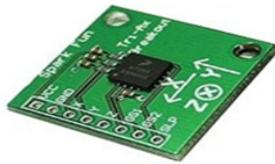
Gambar 6. Board Sensor MMA7260Q
