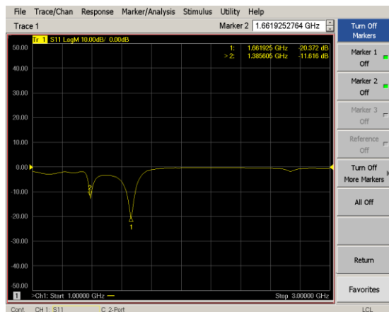
Gambar 9. Pengukuran input return loss (S11) dual band LNA
