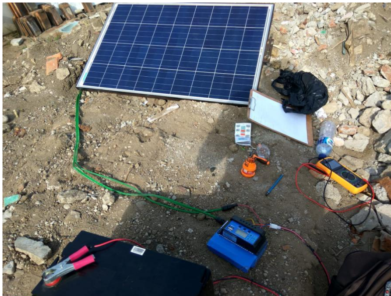
Gambar 7 Pengujian Panel Surya 100 Wp
