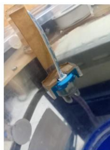
Gambar 18. Implementasi tata letak sensor turbidity
